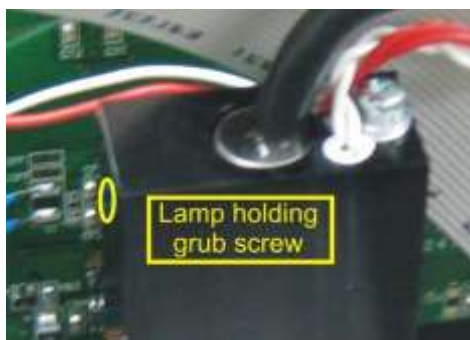
Figure 95 – Location of UV Lamp Fastening Grub Screw
